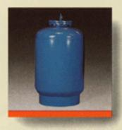
Hydropneumatic Tanks—When desired for maximum energy savings, Hydropneumatic tanks are supplied, either system mounted or for remote installation. Tanks are intended to provide pressure to the installation during periods of low demand so that the booster can be completely shut down, conserving energy and minimizing operating costs.
