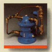
Pressure Regulating Valves—When dictated by the requirements of the installation, pressure regulating valves (PRV's) are used to maintain, precisely, constant downstream pressure regardless of varying suction conditions. Specially sized angle type valves are used to minimize pressure losses and required loads.
